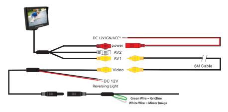
\*Please note: This DC 12V IGN/ACC cable MUST be directly connected to a 12V Ignition Feed.
