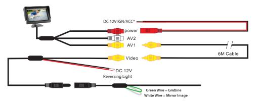
\*Please note: This DC 12V IGN/ACC cable MUST be directly connected to a 12V Ignition Feed.
